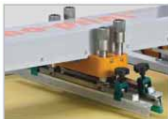
Quick change over of aluminum extruded squeegee and flood bar
